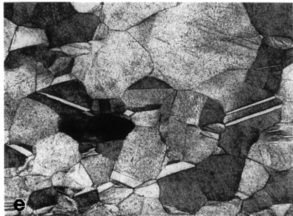
Figure 1 The microstructures developed in pure copper during room temperature tensile testing: (a) in the annealed condition, deformed at a strain rate of 8 \times 10^{-4} /sec to tensile strains of (b) 0.11, and (c) 0.31, deformed at a strain rate of 1.7 \times 10^{-1} /sec to tensile strains of (d) 0.11 and (e) 0.31.
